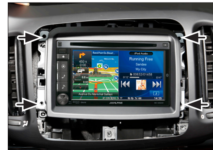
7. Connect all required circuit points Fix double DIN head unit on dashboard (see arrows)
