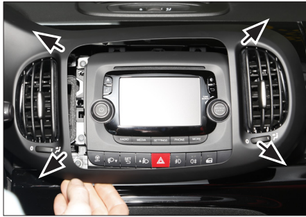
2. Unclip and remove panel carefully (see arrows)
