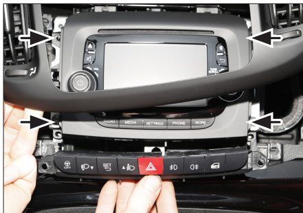
4. Pull hazard light switch bar towards your direction
