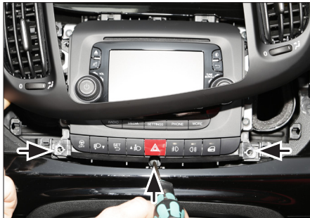
3. Remove 3 screws of hazard light switch bar (see arrows)
