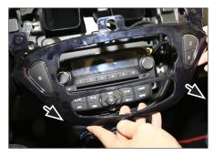
6. Remove OEM cover (unplug all connectors carefully)
