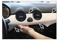
2. Unclip and remove OEM panel
