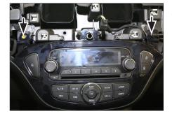
4. Remove 2 screws of head unit cover
