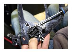
Remove buttons from OEM panel and attach them to new facia plate
