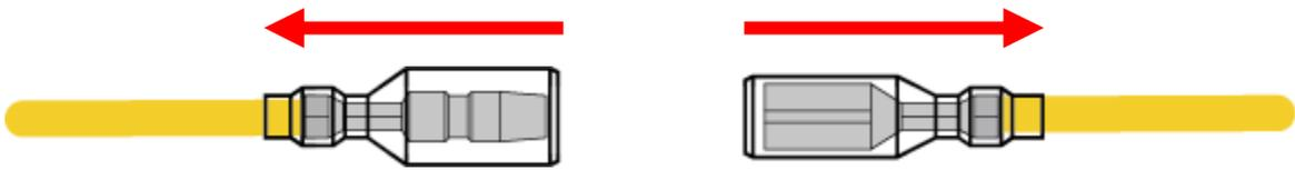
Connect the supplied yellow cable to the cable set and seal the remaining open end with insulating tape.
