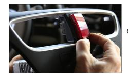
6. Remove hazard light switch from OEM panel
