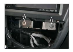
Connect all required circuit points push double DIN head unit into dashboard.
