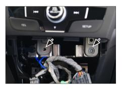
Remove both screws (keep screws, they will be needed later)
