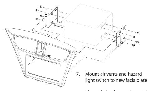
Mount facia plate and mounting brackets to double DIN head unit
