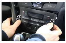
2. Remove air condition control panel (below the radio)
