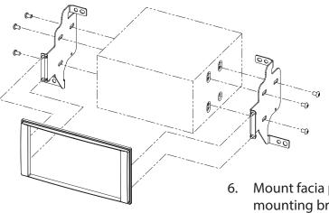
Mount facia plate and mounting brackets to Double DIN head unit
