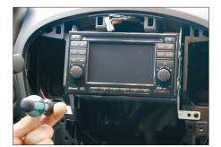
5. Remove screws of OEM head unit
