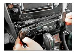
1. Unclip and remove panel under OEM head unit
