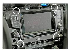
4. Insert radio release keys Remove OEM head unit
