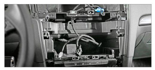
b) Cut plastic bridge underneath removed plastic (see arrows)
