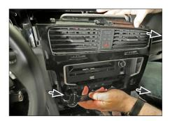
3. Unclip air vents (specail VW tool may be required)
