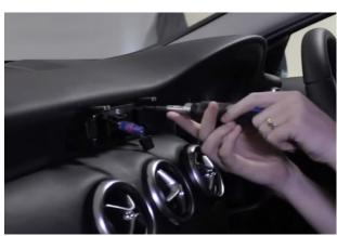
Remove the screws (x2) that hold the main display bracket in place and remove it completely. These top display components can now be stored as they will no longer be needed.
