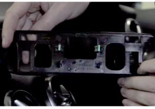
Using a panel removal tool, pry away the top display mounting bracket and fully remove this from the dashboard.
