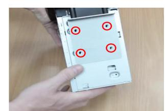
Take the fascia (with brackets attached) and slide this over the new stereo. Align the unit correctly and screw into place (screws not included).
