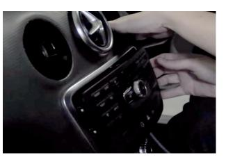
With the screws removed, proceed to pull the main head unit out of the dashboard and remove all of the wiring in the process.
