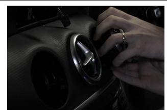
Remove both left & right vents from the dashboard. Undo the screws (x2) that are uncovered by these vents, these screws hold the main head unit in place.
