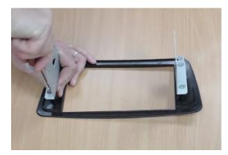
Take the brackets & screws that come within the kit and attach them to either side of the new double din fascia.
