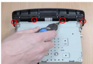
Before putting the main head unit into storage, undo the screws highlighted (x4). This will separate the hazard switch panel which will be used later in the installation (including the screws).
