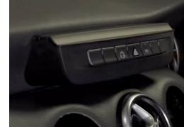
With the mounting bracket attached, grab the hazard switch button panel and proceed to connect to the 'extension wiring'.
