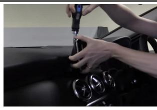
Begin by removing the screws (x2) located behind the top display. Once done, firmly pull the display forward and up from the dashboard.
