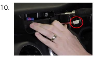
Attach the 'hazard button extension wiring' to the pre-existing connection. Once done, thread this up through the top display port.
