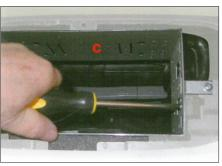
Locate the cage (C) in position, ensuring correct alignment to the foam block and fix it as shown
