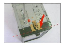
Apply the springs (D) to the 2-DIN Navigation using the mounting hardware (D) as neccessary
