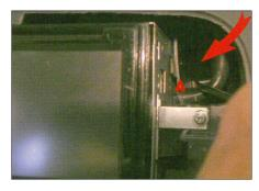
7. Using a screwdriver, or similar push the paddles (A) against the sides of the 2-DIN Navigation to ensure correct air flow from the ventilation ducts
