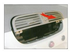
Remove the original Radio and air vent cover
