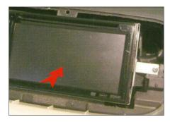
6. Insert the 2-DIN Navigation into the cage until the springs click and engage fully
