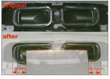
2. Without removing it, cut the front of the air vent duct as shown. It is recommended to offer the cage to the opening to check the measurement befor the final cut!
