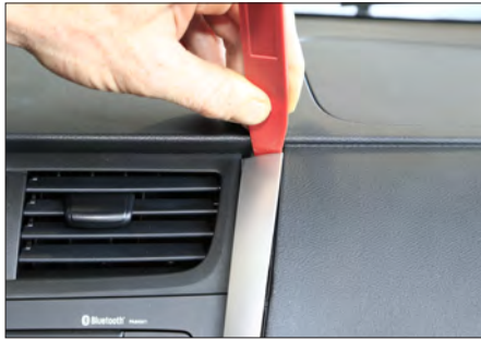
2. Unclip OEM panel carefully
