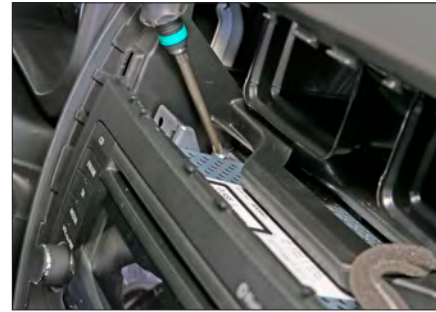
6. Remove 2 screws of OEM
