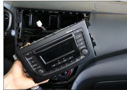
7. Unclip all connectors Remove OEM head unit
