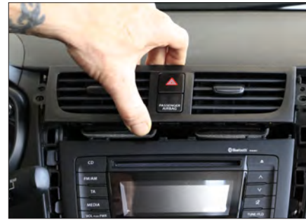
5. Remove air vents Unplug connectors carefully
