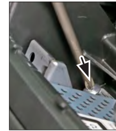
6. Remove 2 screws of OEM
