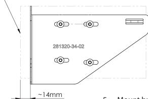
Mount brackets to Double-DIN head unit as shown in the drawing
