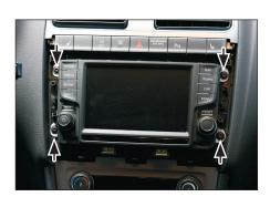
Remove screws of OEM head unit (see arrows)
