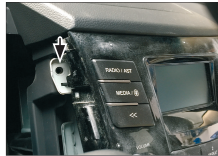
6. Remove screws of OEM head unit
