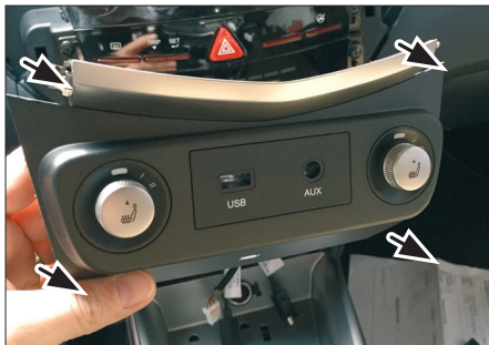
3. Remove air usb panel
