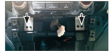
6. Remove screws of OEM head unit
