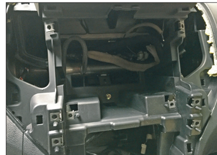
7. Unplug all cables carefully Remove OEM head unit by pulling it into your direction
