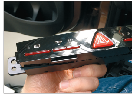
5. Remove hazard light switch
