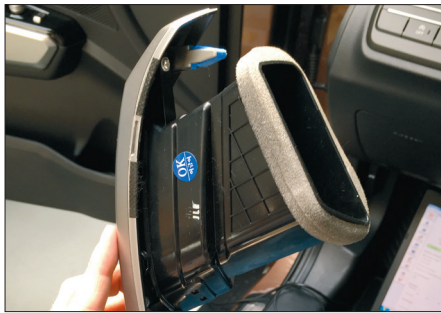
2. Unclip and remove air vent panels
