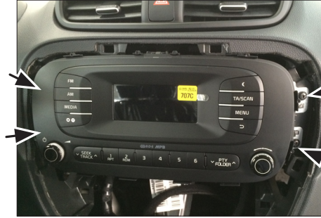
3. Remove all screws of OEM head unit
