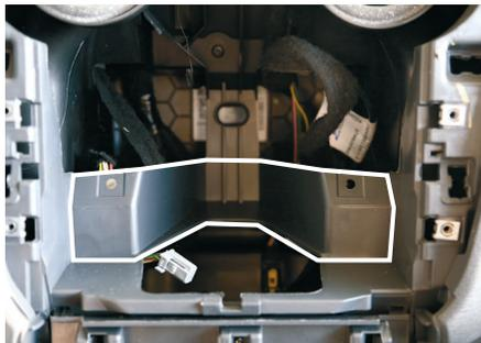
8. If necessary cut plastic in order to clear space for 2-DIN head unit
