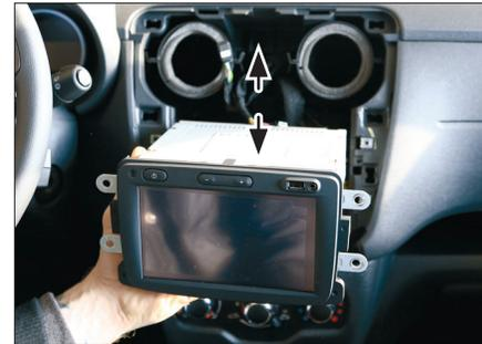
6. Remove OEM head unit (unplug all cables and connectors carefully)
