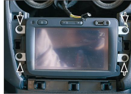
5. Remove 4 screws of OEM head unit (see arrows)
