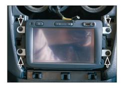
Remove 4 screws of OEM head unit (see arrows)
