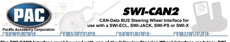
The SWI-CAN2 Interface must be used with one of the following Steering Wheel Interface modules: SWI-ECL2, SWI-JACK, SWI-PS or SWI-X. This Interface will interpret the SWC commands sent on a CAN data BUS and output an analog signal which is then used by the SWI-ECL2, SWI-JACK, SWI-PS, or SWI-X to control your aftermarket radio.
