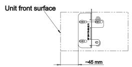
We recommend a distance about 45 mm to the front surface of the 2-DIN head unit
