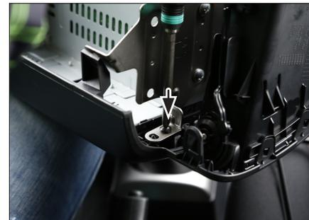
7. remove all screws holding the OEM head unit in center console
