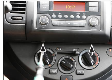
5. Remove screws under OEM head unit (see arrows)
