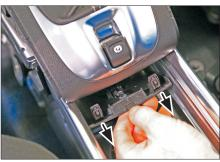
4. Unclip and remove panel under the gear box (see arrows)
