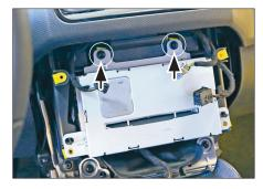
7. Remove two screws of OEM head unit
