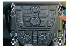
3. Remove 4 screws of OEM front panel (see arrows)
