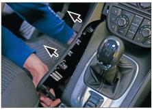
2. Unclip und remove side panels at the left and right side
