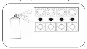
4. Fold the cardbox template into a box. Spray paint the sensors and the adapters and let dry thoroughly before assembling. **NB**: Too much spray paint can impair the sensors performance.
