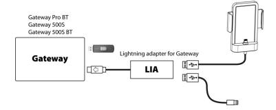
Installation and usage of the LIA to retain the USB flash drive capability. (with DAB+G)
