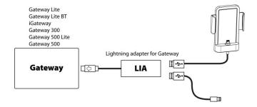
Installation and usage of the LIA to retain the USB flash drive capability. (without DAB+G)
