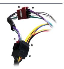
7. Connect the female vehicle specific connector to the male vehicle connector. Test head unit for correct operation.
