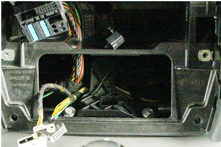
5. Loosen the two screws at the bottom of the plastic frame. Remove the plastic frame from the center console. This is, except for reassembly of the CD original device, in the course no longer needed.
