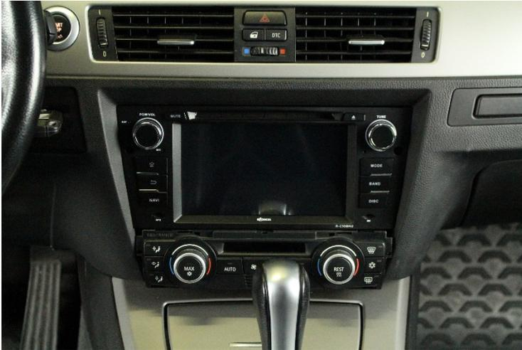
9. Connect the two remaining plugs to the climate control panel. Close the locking mechanism of both connectors. Align the climate control panel in front of its intended position and press it in place.
