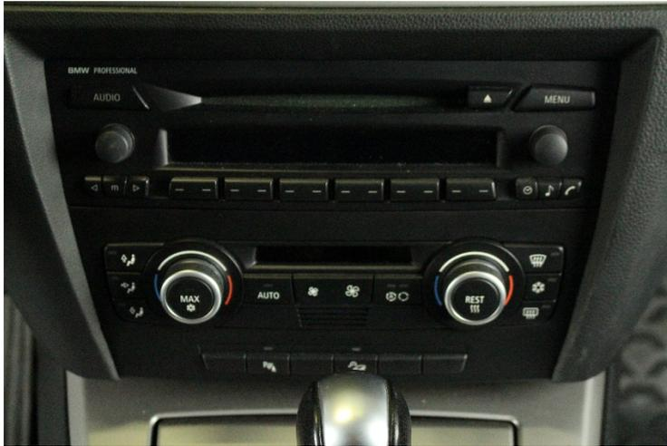
1. Unlock the automatic AC control panel out of the center console with the unlock tool (No. 10) contained in the set.
