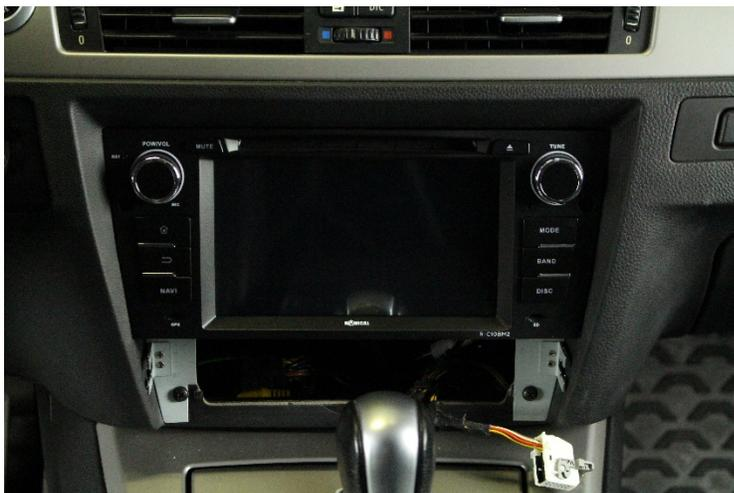
8. Install the two supplied mounting frames made of metal (No. 17/18) with the two original screws in the mounting slot. Connect all cables previously routed in the radio slot and the original antenna cables to the Radical unit (No. 1). Carefully insert the R-C10BM2 into the bay and secure the unit with the two screws provided with the hardware accessory set.
