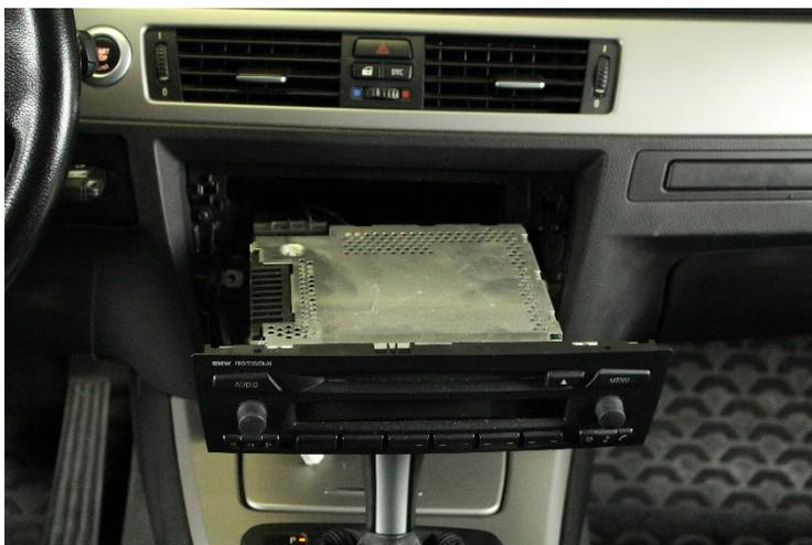
3. Loosen up both screws underneath the factory installed CD radio. Pull the unit out of the center console. Open the locking lever of the Quadlock connector and unplug all other connectors and cables such as FM antenna lead, etc. Put the OE CD radio to the side in a safe place, to protect it from damage.
