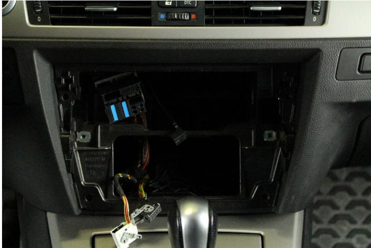
4. Remove the four screws that fix the inner plastic frame to the mounting slot. Pull the plastic frame out of the center console. This frame will be of no more use, except for a later reinstallation of the original CD unit.
