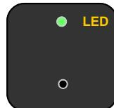
Now press 3 times the module button, the LED will flash RED (UNITS), GREEN (TENS) and YELLOW (HUNDREDS) flashing.
