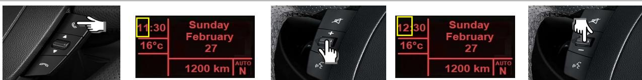
To turn to the MINUTES setting, press PHONE ANSWER. Volume buttons allow MINUTES adjustment. In this example is 11:30.
