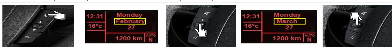
To turn to the DATE setting, press PHONE ANSWER. Volume buttons allow DATE adjustment. In this example the DATE is 27.
