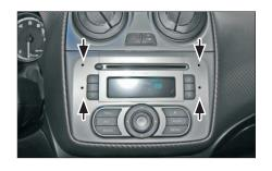
Insert special radio release keys in the holes of the OEM Radio
