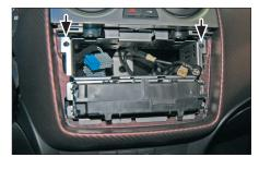
3. Remove the original metal holder inside the the dashboard, which is fixed by 2 screws (see arrows)
