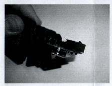
During this operation, adjust the distance between the two PCB, in order to facilitate the insertion of the part.
