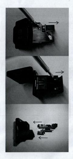
Take the original part and, in order to unhook the rear plastic, use a screwer by lightly pressing into the slots as shown in the picture.
