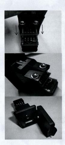
Screw through the PCB until you get a good fixing of the board to the plastic case.
