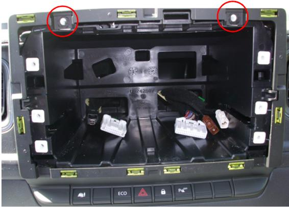
*After removing the radio tighten the screws again.*
