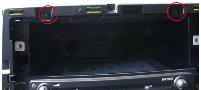
*Remove the marked screws and bend the frame slightly forward. Now the radio can be removed.*
