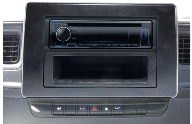
If all screws have been tightened again, the cover plate can now be finally fitted. You should hear clearly any click from the noses on the backside. Built in the metal frame from the new radio and install the radio.
