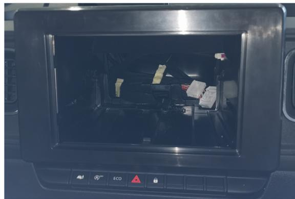
*Hold the cover plate over the metal frame, but do not press it on and snap it into place. Check if the metal frame is located centrally behind the cover panel, if not, move it in place. Remove the cover plate again and tighten the screws.*
