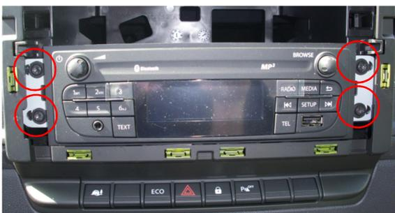
*Remove the screws from the factory radio.*
