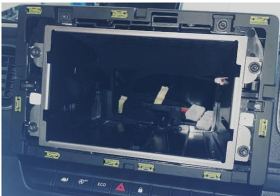
*Fit the metal bracket but do not tighten the screws yet.*
