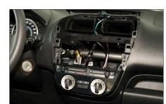
6. Dashboard with removed OEM head unit
