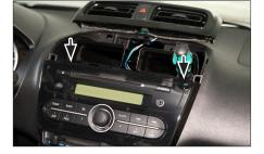
4. Remove two screws of OEM head unit (see arrows)
