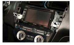
Connect all required circuit points. Place double DIN Navigaton on dashboard and fix it with two screws (see arrows)
