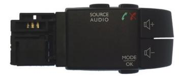
This interface is designed for the above stalk paddle. The SOURCE AUDIO button will change source, the phone button will answer (short press and reject (long press) calls. The volumes buttons increase and decrease volume, the MODE OK button skips through presets and the scroll wheel on the back of the paddle skips tracks back and forward.
