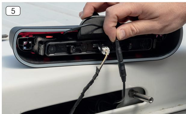
5. Connect the 3.5 mm jack output of the camera sensor to the black counterpart on the main wire and wrap around some isolating tape around it to prevent water entering the connector
