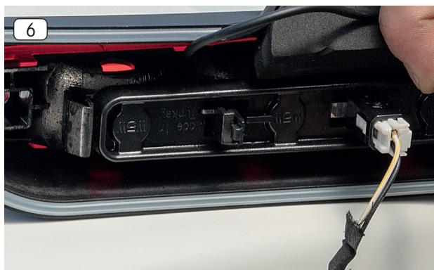
6. Connect the system plug with the connector counterpart of the brake light reflector housing.
