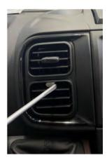
Loosen the 4 screws from the frame
