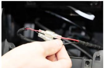
Connect the additional cables and insert the CARica into the recess of the original storage compartment. First insert the rear side with the guide pins.
