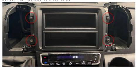
Remove the frame with the pockets or remove the radio
