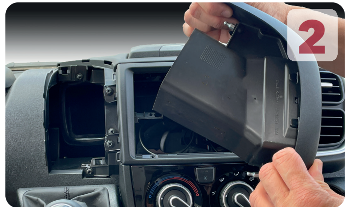
2 Remove the airvents left an right by pulling They are attached with two pins
