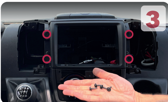
3 Remove four screws using a T20 screwdriver Keep them a side for later
