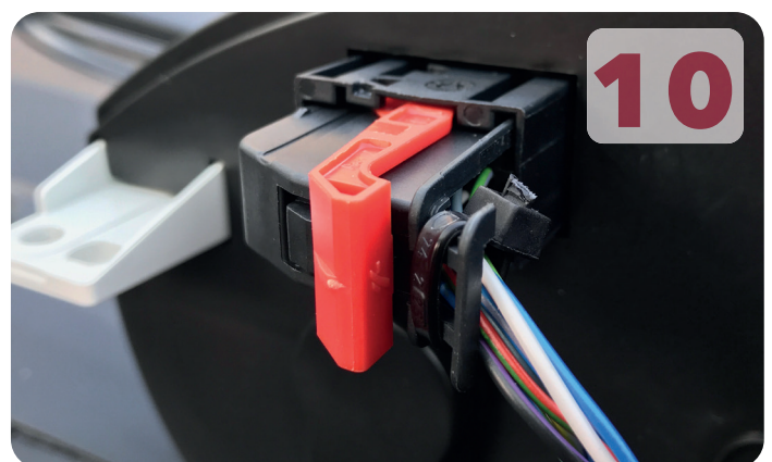
Remove the connector by sliding the red tab away from the cables
