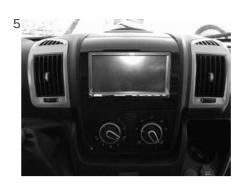
5 Connect all cables, verify the proper functioning of the system and insert the radio-frame into the housing. This is the final result.
