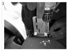
3 Put the mounting brackets on the new facia plate provided and fix them with screws. Pay attention to the letters on the brackets.
