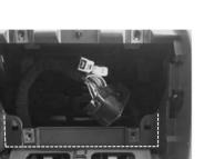
2 Cut and remove the plastic parts along the dotted white line in the figure.
