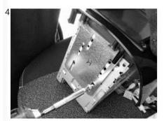
4 Take the AFT unit and fix it to the assembly with screws.
