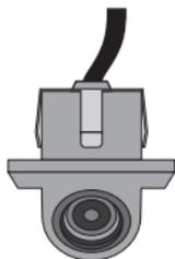
Flush: Drill a 22,5mm hole into the right place and press the camera carefully into the hole.
