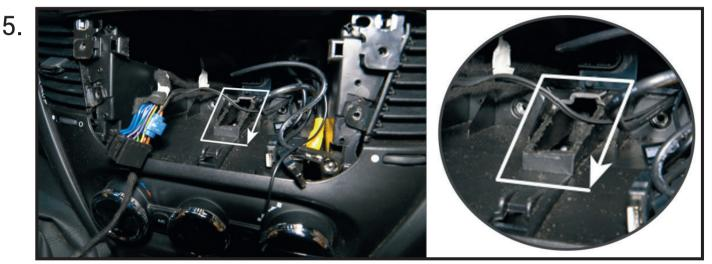
The highlighted sections of the dashboard will need to be cut in order for the new head unit to sit in place correctly.
