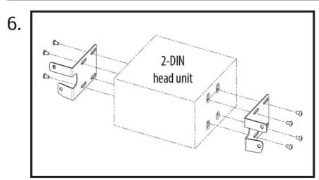
Take the brackets from the kit and attach them to the correct sides of the new head unit.
