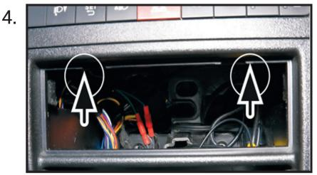
Proceed to then remove 2x screws that are located up within trim of the main fascia. Once undone, pull the fascia away from the dashboard.
