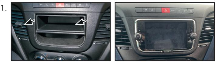
Start by using a panel removal tool to remove the pocket from the front of the fascia.
