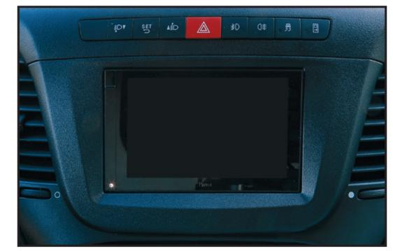
With the head unit in place, proceed to fit the new fascia panel over the front of the radio to complete the installation.
