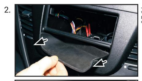
Just below the pocket will be an aperture with an anti-slip mat. This will be fixed in place with double-sided tape/glue. Pry this out of the dash.
