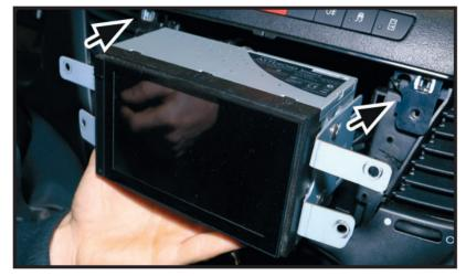
Once the head unit has been wired up correctly, proceed to slide the head unit into the dashboard. At this point, it would be best to test fit the stereo to ensure the wiring is correct.
