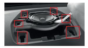
The original speaker is plugged in at three points on the panel. If necessary, use a plastic wedge to lever out the speaker. To unlock the connectors, use either a small screwdriver or a paper clip. Connect the supplied crossover to the original connection cable (gray / gray black) and the other end to one of the two connection terminals of the EM-MBC1.
