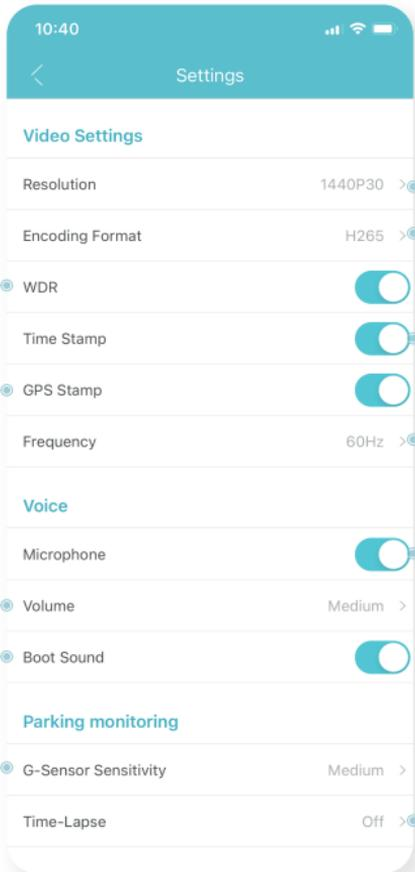
The image shows a smartphone settings screen for the DC102 device. The screen is titled 'Settings' and has a teal header. The settings are organized into sections: 'Video Settings', 'Voice', and 'Parking monitoring'. Each setting has a radio button, a toggle switch, or a chevron icon. Blue lines connect text annotations to specific settings on the screen.
