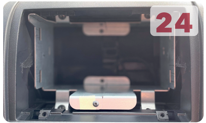
Final look of the mounting cage in the dashboard
