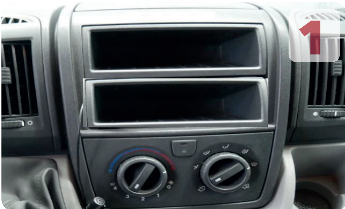
Original dashboard setup Remove the storage pockets
