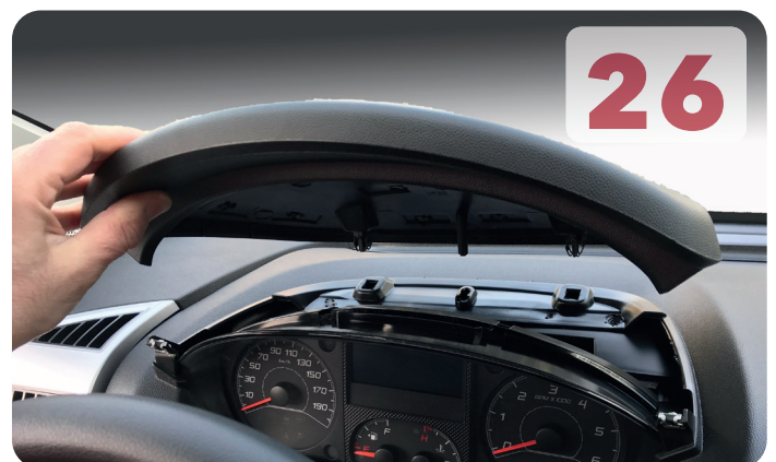
Remove the tacho visor It is still secured with clips
