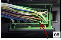
The speed signal is located as shown in the picture. Please only choose 1 connection point: either in the Black connector, pin 22, or in the Green connector, pin 04.
