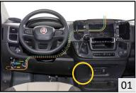
Routing of the speed & reverse cable an position of Grey connector (3)
