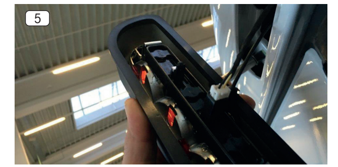
5. Insert the brake light assembly into the main housing. Next, plug in the white power supply system connector into the socket on the brake light reflector housing backside. Connect the mini-4PIN connector of the cam sensor end to its counterpart of the extension cable.
