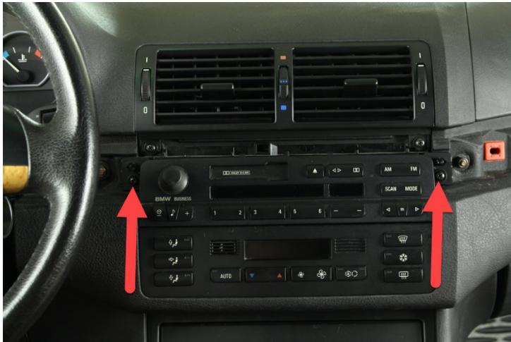
4. Use a Phillips screwdriver, loosen the two side fixing screws of the OE radio.
