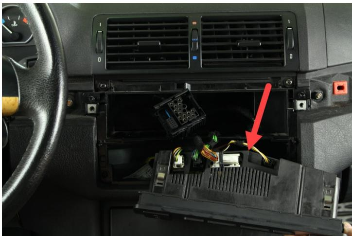
6. Release the AC control unit from the center console by pressing from behind and disconnect all connections at the backside of the air conditioning control unit.
