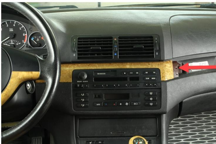
3. Unlock the trim above the radio with the plastic unlock tool (Nr. 10). To do this, you must place the plastic removal tool on the side and carefully pry out the trim strip.
