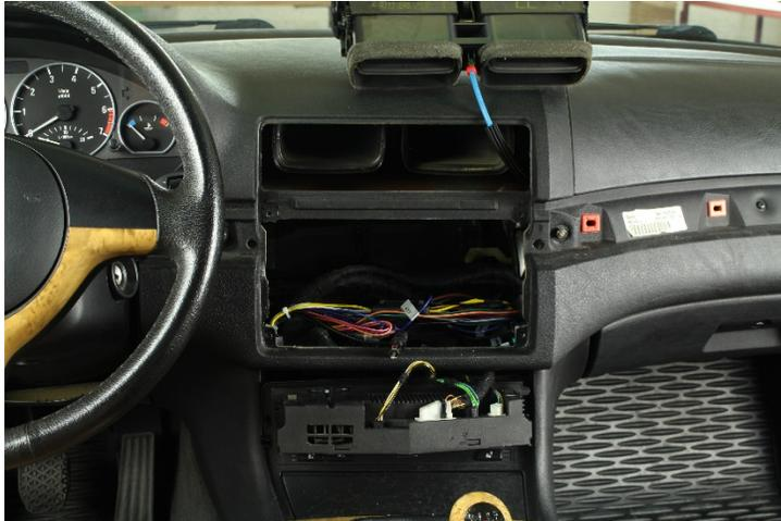
10. Route the connections of the AC control unit through the opening of the previously removed storage compartment and connect the connections to the climate control unit.
