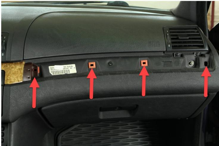
2. To do this, place the plastic removal tool at the marked points from below on the trim strip and then carefully pry it out.
