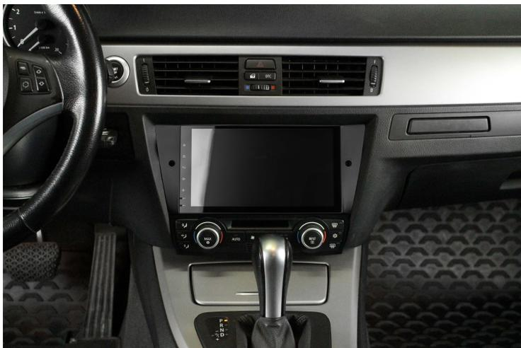
10. Connect the appropriate plastic frame supplied with the climate control unit.
