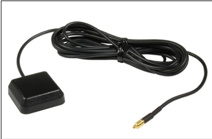
6. Install the GPS antenna (No. 2) in a suitable position, making sure that the GPS reception is not adversely affected by unwanted shielding of metallic vehicle parts (thermal insulation glazing, etc.). Then route the connection cable into the radio bay.
