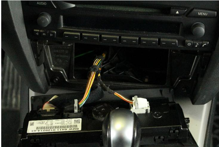
2. Pull the AC control panel out of the slot and release the latches of the connectors on the backside. Now detach the AC control panel and car specific optional button assembly from the mounting frame. Keep the AC control panel and the car specific button assembly within reach, for later reassembly.
