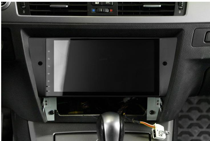
8. Install the two supplied mounting frames made of metal (No. 17/18) with the two original screws in the mounting slot. Connect all cables previously routed in the radio slot and the original antenna cables to the Radical unit (No. 1). Carefully insert the R-C11BM2 into the bay and secure the unit with the two screws provided with the hardware accessory set.
