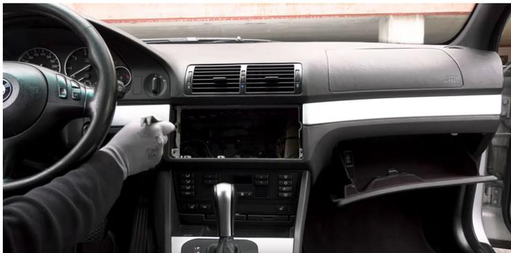
3 Take the supplied release tool (# 10), and loosen the two plastic panels at the top of the shaft.
