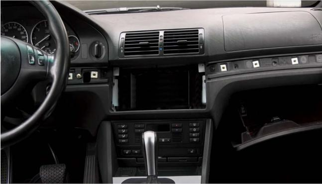
1 Now take the supplied mounting bracket (No. 15) and place it in the radio slot. Screw these tightly with the Phillips screwdriver on the inside of the shaft.
