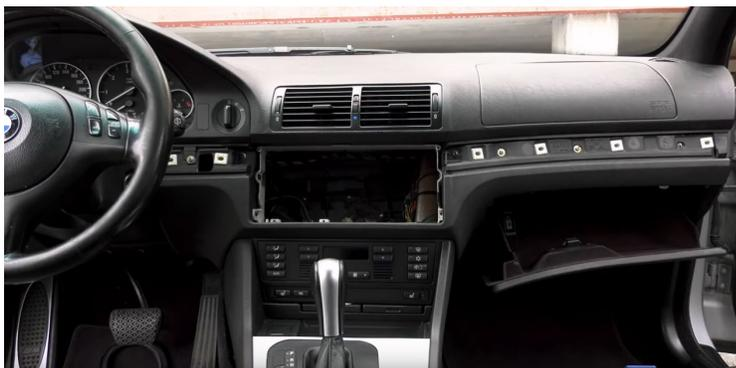
4 Use a Phillips screwdriver to loosen all connecting screws of the center console (see picture), depending on your model.
