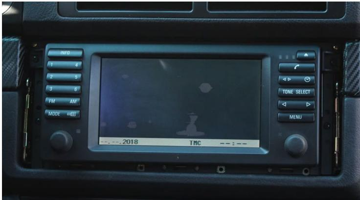
1 Use the supplied release tool (# 10) to release the trim frame. Then remove the screws connected to the center console.
