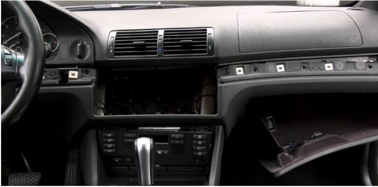
5 To be able to remove the metallic radio bracket from the shaft, you must now loosen all the screws connected to the center console, left and right in the glove box. Only then can you
