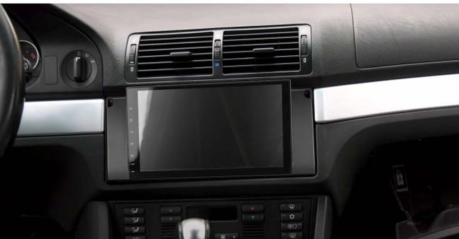
3 Carefully lay the various connection cables of the Radical device in the lower area of the radio shaft. Fix the device firmly to the center console with the two supplied screws. Reinstall all the screws you loosened previously and turn them tight. Then attach the plastic panels back to their usual place.
