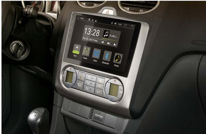
4. Neatly arrange the wires to the side, making room for the Radical device. Carefully slide it into the radio slot. Push back the R-C10FD2 until you hear the clicking sound of the latching mechanism.
