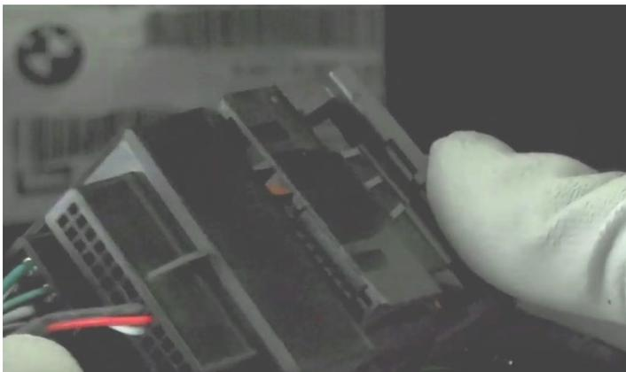
3. Connect one of the main connection cables (No. 11) of the Radical device (No. 1) to the Plug connector of the car and close its locking mechanism. Following this, connect the CAN bus interface (No. 12) to the main connection cable. Connect all the cables inside the radio bay and the original antenna cables.
