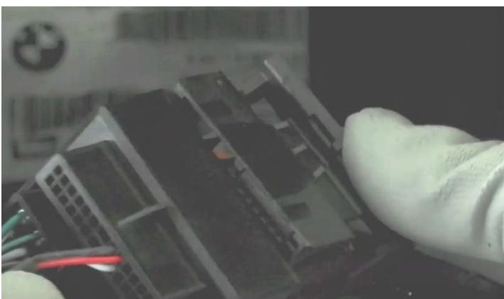
10. Connect the respective main connection cable (No. 11) of the Radical device (No. 1) to the plug of the vehicle and close the locking mechanism of the plug. Then connect the CAN-BUS interface (No. 12) with the main connection cable. Connect all the cables previously laid in the radio slot and the original antenna cables to the Radical device (No. 1).
