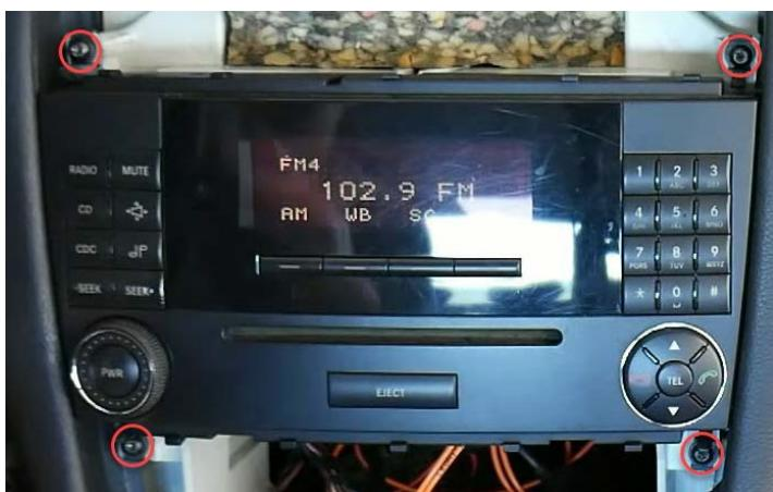
6. Then remove the four retaining screws of the original radio.
