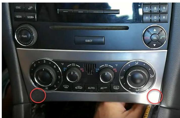
3. Now you have to loosen the brackets for the cover in the center console. For this you need a thin, long slotted screwdriver. After you have loosened the clips, you can pull all the plugs off the controls.
