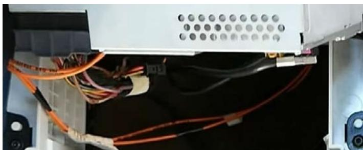
7. Carefully pull the original radio out of the shaft at the necessary speed. Make sure that you do not damage the cables. Remove the cables one at a time and carefully, make sure that the cables do not fall back into the slot.
